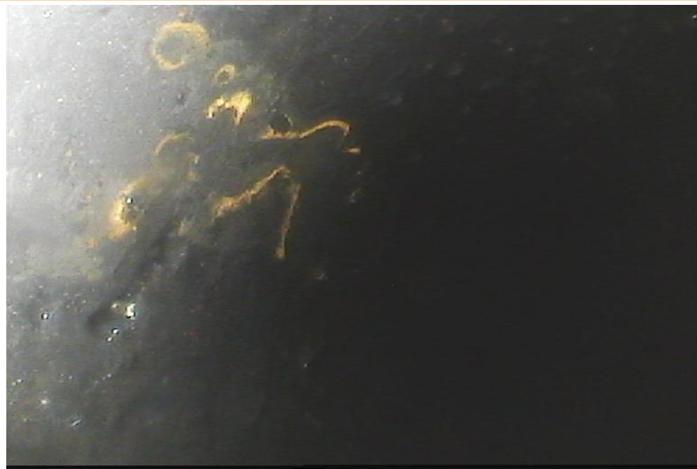
Tube No:112-Fault: Pitting >40%
