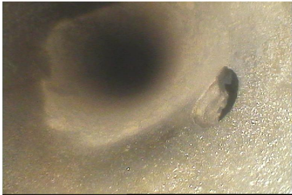
Tube No:112-Fault: Pitting >40%
